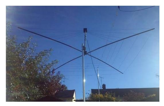
Much of the inspiration (not to mention technical details) was obtained from <u>G3TXQ's CobWeb</u> <u>webpage</u>. The antenna compliments my 40m dipole nicely and gives me the most useful HF bands (40-10m) without needing an ATU. Note the spelling of CobWebb vs CobWeb – The original G3TPW was designed by Steve Webb, hence the spelling. As this is the G3TXQ variant, I refer to mine from now on as a "CobWeb".
